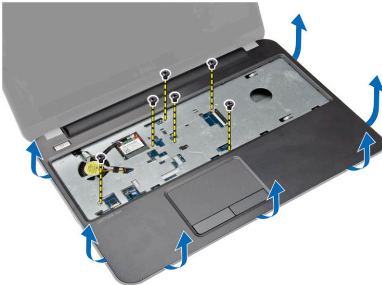
6. Lift the palmrest at 45-degree angle and remove it from the computer.
