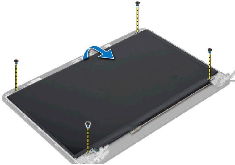
4. Peel the tape that secures display cable and disconnect the cable from the connector. Remove the display panel from the display assembly.
