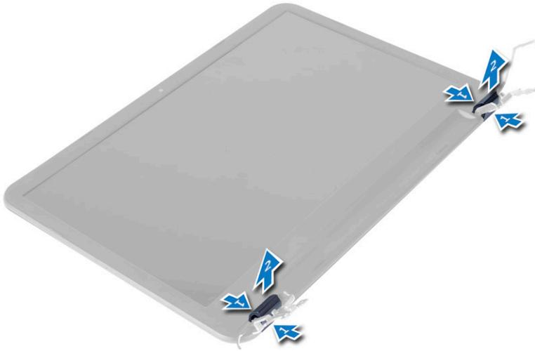
4. Pry the edges of the display bezel. Remove the display bezel from the computer.
