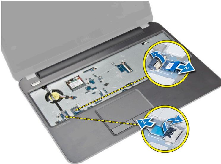
5. Remove the screws that secure the palmrest to the system board. Lift and release the tabs on palmrest from the slots on the computer.
