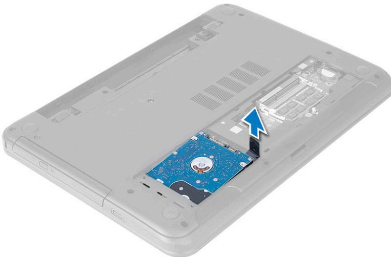
5. Remove the screws that secure the hard-drive bracket. Lift the latch to remove the hard-drive bracket from the hard drive.
