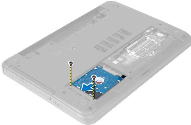
4. Slide the hard drive to release it from its connector. Lift the tab to remove the hard drive from the computer.
