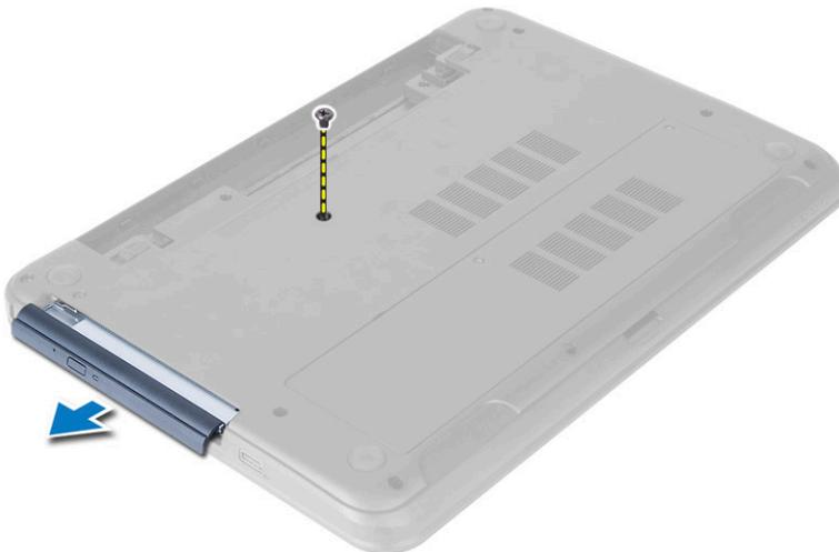
4. Remove the screws that secure the optical-drive bracket to the optical drive. Remove the optical-drive bracket from the optical drive.
