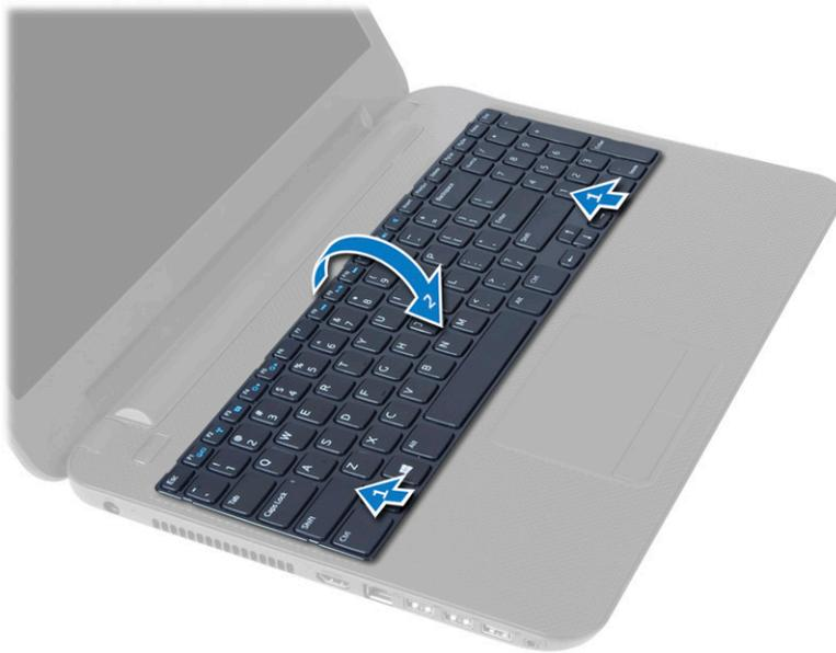
5. Disconnect the keyboard cable from the connector on the system board and lift the keyboard off the palmrest.
