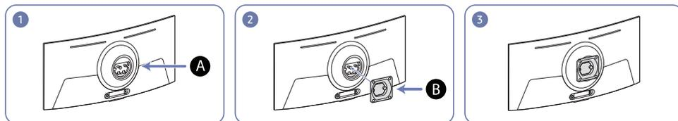
**A** Attach the BRACKET WALL here
