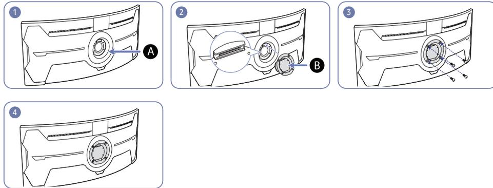
**A** Attach the BRACKET WALL here
